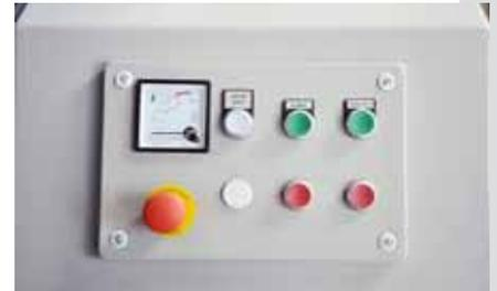
To minimize the needed floor space and make the machine easy to move, machine controls and electrical cabinet are integrated into the machines soundproof housing.
