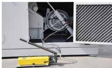
To ensure a safe operation and quick and easy access for cleaning and maintenance the GSC 500 machines cutting chamber is opened hydraulically.
