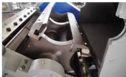
The GSE granulators are available with different rotor options to fit different applications, all rotors feature the V-cut technology creating a high quality regrind.
