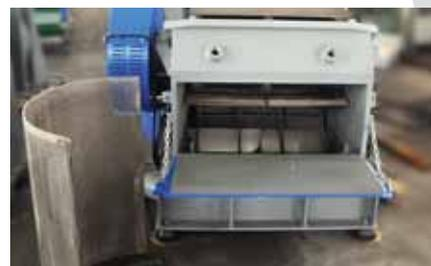
The redesigned base of the GSE 700 series makes the machine very sturdy, while maintaining the easy accessibility for maintenance and cleaning.
