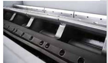
The GSH 1100 series comes standard with wide H-style rotors available with 9, 11 or 13 rows of rotor blades ensuring a high quality output.
