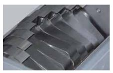
Staggered rotor blades creates an individual blade cut thus increasing the cutting torque. All of the machines in this series are therefore suitable for grinding more solid materials and thicker walled sprues.
