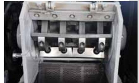
The cutting chamber sits in a soundproofed enclosure to ensure quiet inline operation. The rotor and screen area are easily accessible without for cleaning and maintenance.
