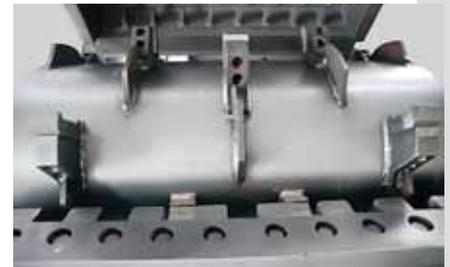
The combination of pre breakers and counter knives create a high impact powers resulting in a high degree of disintegration and high throughput rates.
