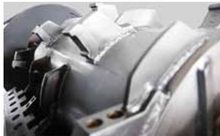
The ZHM hammer mill features a flat rotor with innovative welded tool holders. This heavy duty rotor design ensures a smooth operation on various materials.
